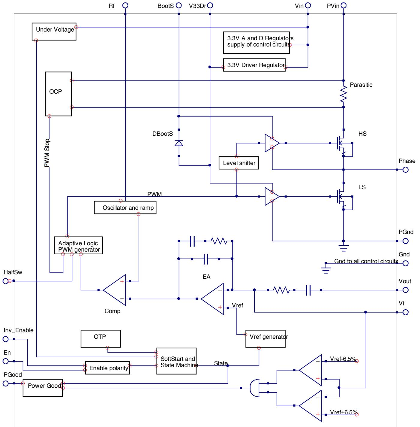
Figure 2: Block diagram of the FEAST2 ASIC.
