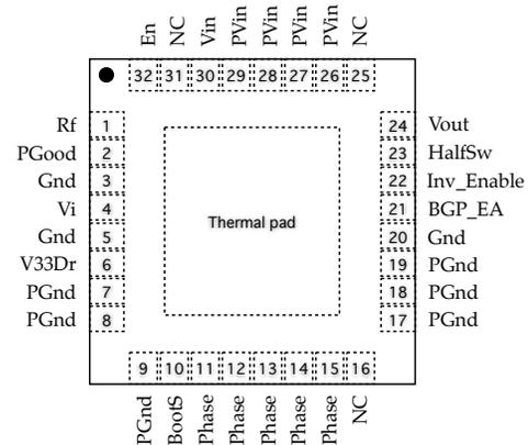
Top view - 32-lead plastic QFN (5x5 mm)
