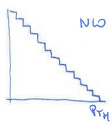
The integral is the NLO cross section; the virtual contributions to the first bin and its large negative contribution compensates the positive divergent contribution of the real. However the differential cross section has an unphysical behavior at  $P_T \rightarrow 0$ . This divergent
