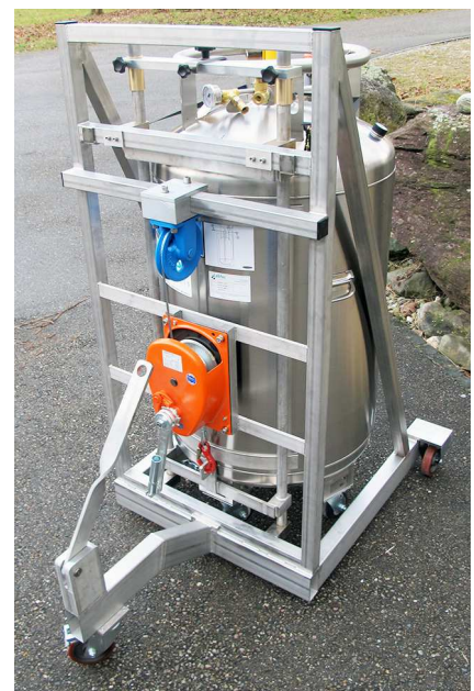
- Liquid nitrogen vessel transfer car
