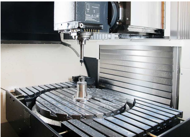
- The 1250 mm x 700 mm work area with 70 cm rotary table
