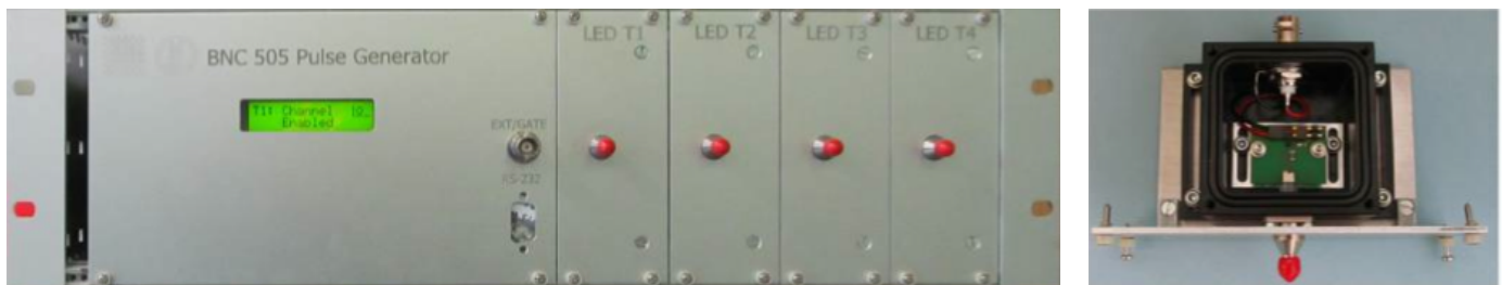
FIG. 4.4 – LED modules and matching pulse generator designed by our technician A. James. The picture on the right shows the light-tight enclosure inside an LED module. The light output is provided through an optical SMA connector.
