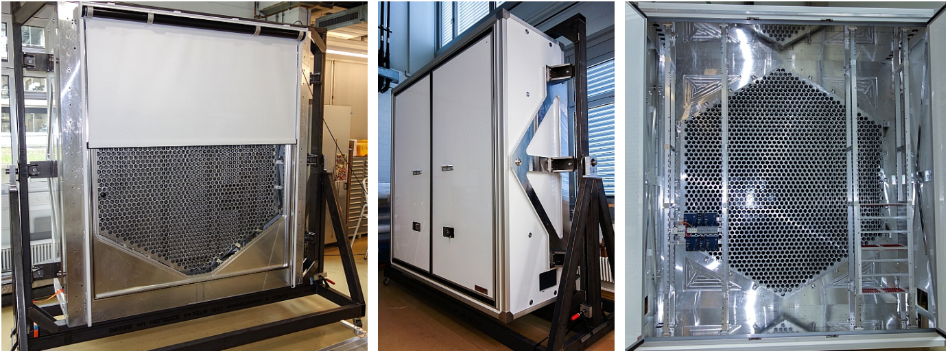
FIG. 7.2 – Pictures of the camera body. From left to right: front view with half closed lid, rear view with closed doors and rear view with open doors showing the two electronic racks.
