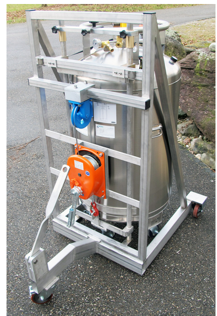
- Liquid nitrogen vessel transfer car
