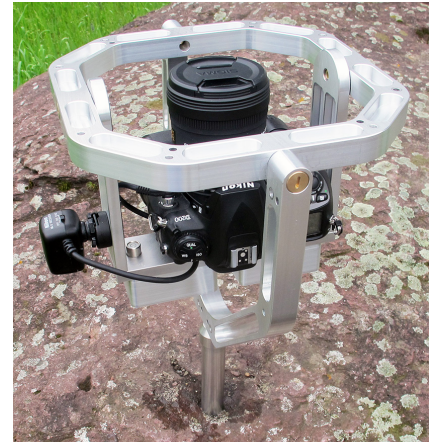
- The gimbal camera suspension
