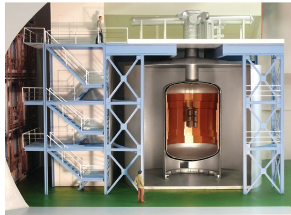
Fig. 3.1 – Mock-up of the GERDA setup situated underground at LNGS. Currently, a string with three natural Ge-detectors is inside the cryostat. Enriched ^{76}\text{Ge} detectors are installed this year.
