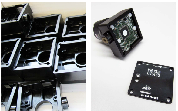
Fig. 17.12 – Left: plastic camera housings. Right: complete opened camera.
