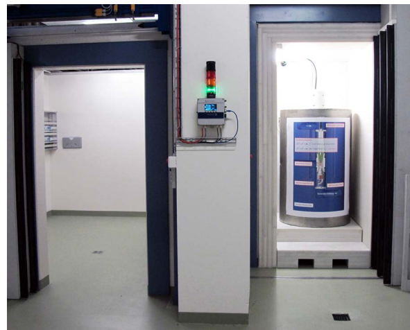
Fig. 17.8 – Neutron generator installed in the shielding compartment. The fusion neutron source is mounted in the vessel to the right.
