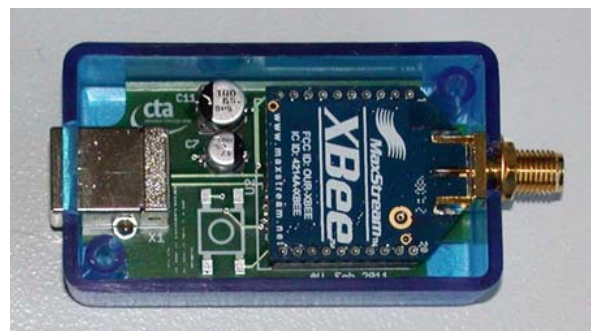
Fig. 18.3 – AMC master controller unit.
