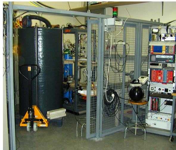
Figure 1.12: Installation in the laboratory showing the 1600 kg cylindrical shielding (grey) made of water extended polyester (WEP) mixed with a boron absorber (Colemanite, \text{CaB}_3\text{O}_4(\text{OH})_3 \cdot \text{H}_2\text{O} ).
