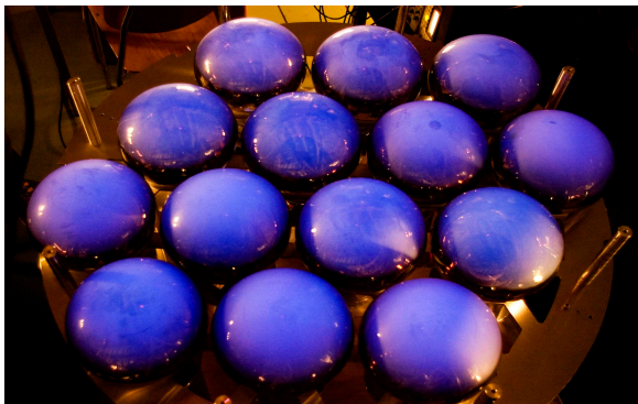
Figure 1.9: The 14 cryogenic PMTs coated with WLS, ready to be installed at the bottom of the ArDM apparatus, illuminated with UV light.
