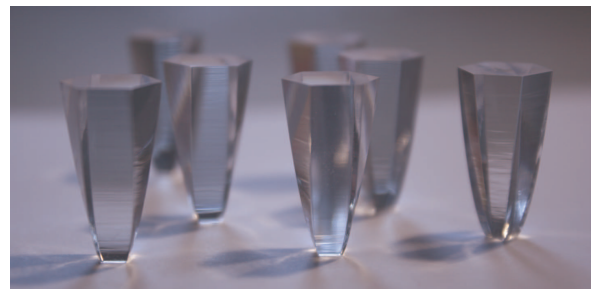
Figure 5.6: A collection of solid, refracting light concentrators constructed at UZH.
