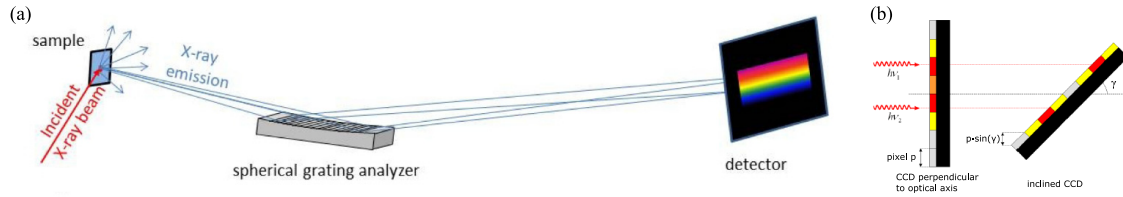
Figure 2.4.: (a) Schematics of a RIXS spectrometer using a spherical grating. Taken from Ref. [32]. (b) Sketch of the spatial resolution improvement by tilting the detector. Adapted from Ref. [33].
