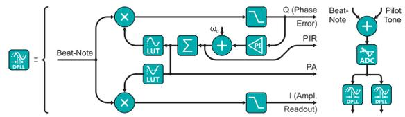
To eliminate relative ADC timing jitter, an analog **pilot tone** is added to each input channel and tracked by a separate DPLL for dynamically resampling the various beat-note signals during post-processing as a part of the time-delay interferometry (TDI) algorithm.
