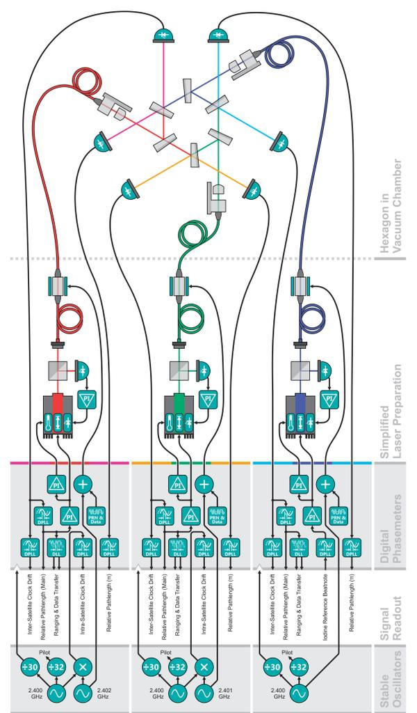
The measurements will be performed by **three fully independent PMSs** connected to each other only via phase modulations imposed onto the three input laser beams.
