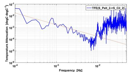
Figure: Transfer function estimation of the cylinder.
