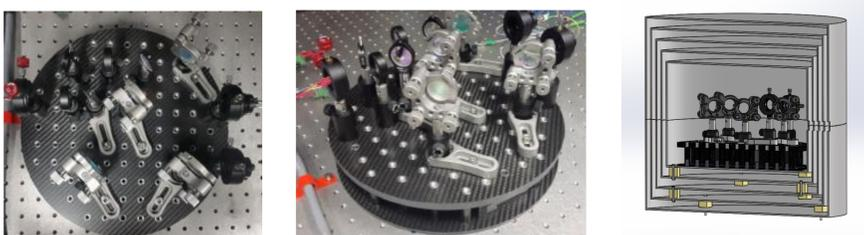
Figure: Mach-Zehnder interferometer assembled on the breadboard.
