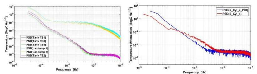
Figure: Temperature noise measured with and without active control. The horizontal line is our read-out noise.
