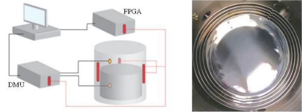
Figure: Scheme of the ultrastable thermal environment and the lower part of the 5 concentric cylinders inside the vacuum chamber.
