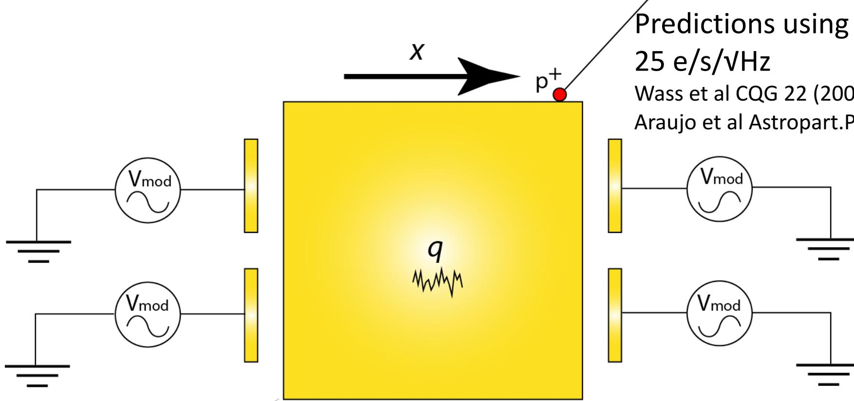
$$\Delta_g = -\frac{1}{m} \left| \frac{\partial C_x}{\partial x} \right| \left( \frac{q_1}{C_{\text{tot}}} V_{\text{mod}} \sin \omega_1 t + \frac{q_2}{C_{\text{tot}}} V_{\text{mod}} \sin \omega_2 t \right)$$
