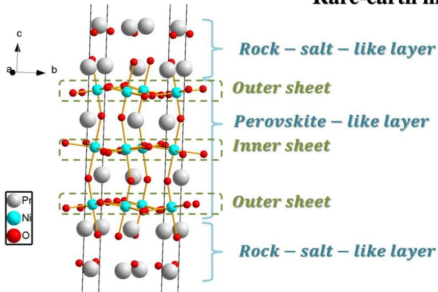
The Ruddlesden–Popper (R-P) rare-earth nickelate  $\text{Pr}_4\text{Ni}_3\text{O}_{10}$  is constituted of infinite perovskite-like quasi-2D layered structures. These layers are connected by  $\text{NiO}_6$  octahedra via shared vertex oxygen ions, and are separated by rock-salt like layers (PrO) along the crystallographic  $c$ -axis. There exist two different types of Ni sites, one in the inner perovskite layers, and the other type in the outer perovskite layers.
