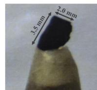
The single-crystal growth of  $\text{Pr}_4\text{Ni}_3\text{O}_{10}$  was performed in an optical-image floating-zone furnace in oxygen atmosphere at 140 bar. The obtained single crystals can be as large as  $3.5 \times 2 \times 0.3 \text{ mm}^3$ .
