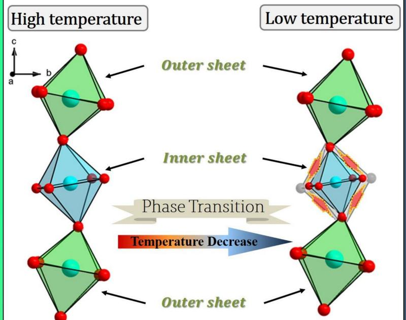
In the low temperature phase, the inner  $\text{NiO}_6$  octahedra shrink as compared to that of the high-temperature phase. However, there are no visible differences between these two phases in the outer  $\text{NiO}_6$  octahedra. This subtle change of the environment of the inner Ni sites must be responsible for the differences in resistivity and magnetization between the high-temperature and the low-temperature phases.
