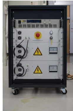
Left: high current coil driver plus differential high gain amplifier for demonstration experiments; Middle: 15 kA current pulser with redundant safety circuit to generate high magnetic fields with small coils for the Chang group; Right: 1.8m radiotelescope on the roof of Y36.
