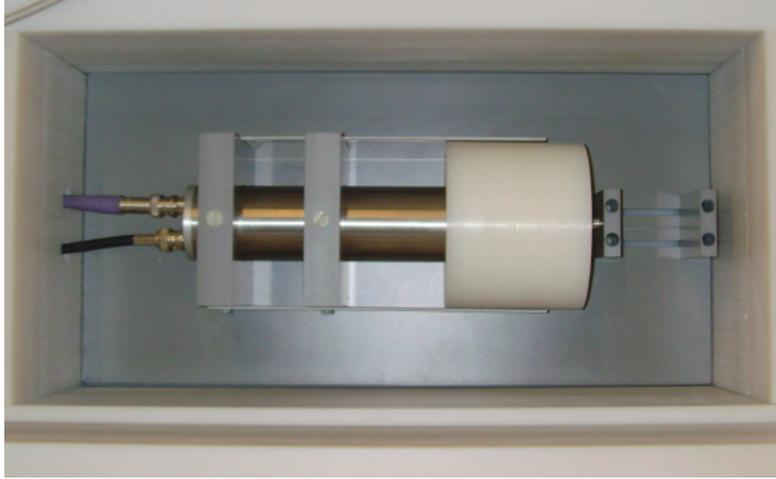
FIGURE 6.10: Photo of the LiI(Eu) neutron detector surrounded by borated polyethylene shield (white). From left to right: SHV high voltage and BNC signal out cables, aluminum housing containing the LiI(Eu) detector (silver), 5 cm polyethylene shielding (white), 2 cm lead brick, and source holder.
