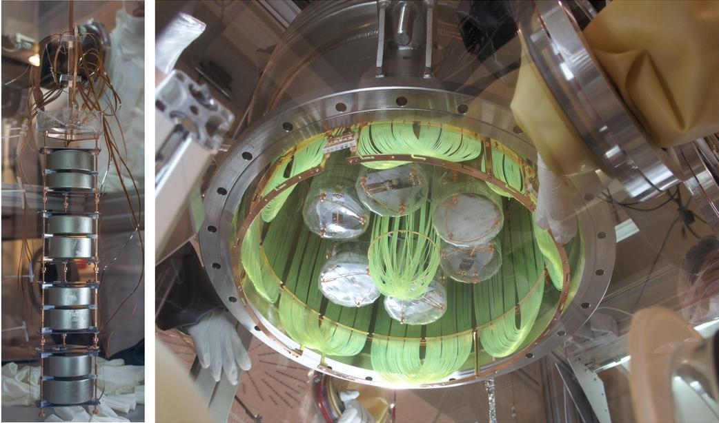
FIGURE 2.2: Photo of GERDA Phase II BEGe detector string (left) and the LAr veto fibre shroud (right) that guides the scintillation light to the Silicon Photomultipliers. The picture is taken after its upgrade in April 2018 to make it denser and thus increase its light yield by a factor two.
