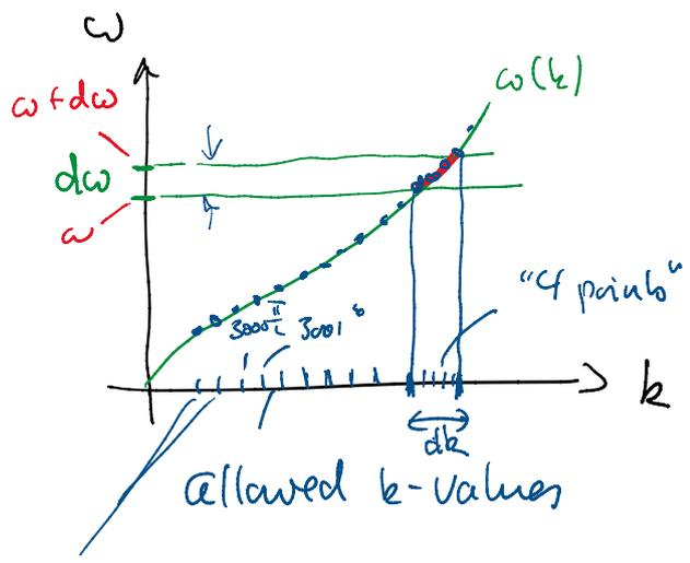
DOS  $g(\omega) d\omega = \# \text{ states in } [\omega, \omega + d\omega]$
