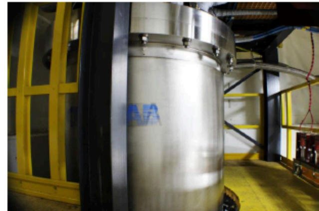
100 Tesla Pulsed magnet
