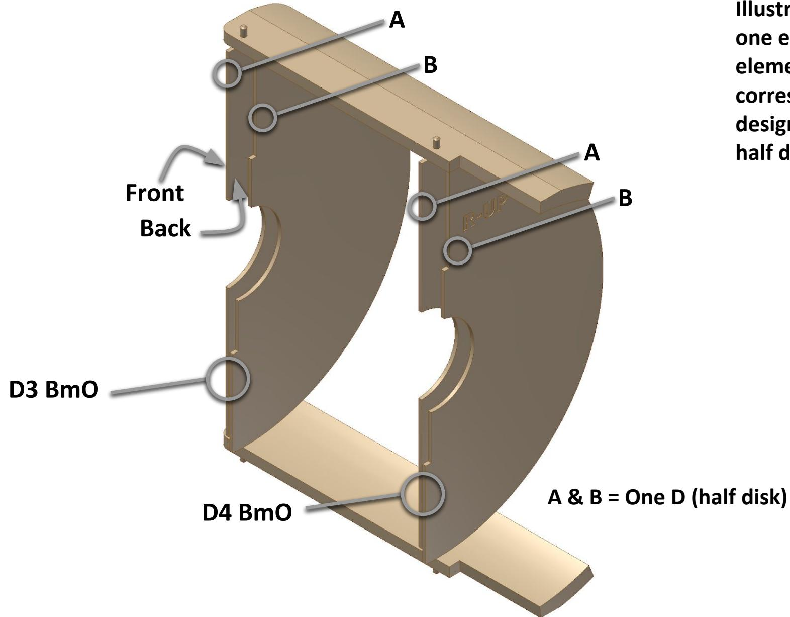
**Illustration shows one ePix detector element with the corresponding designations of the half disks.**
