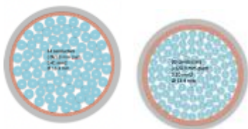
Figure 30 Cables used for the individually wired ‘Grouped’ LpGBT power scheme. On the left, Cable 3 for the LVPS-PP1 part, with 15.3mm outer diameter, can power 42 DC-DC-DC converters. Right, Cable 4 for PP1-PP0 part, with 13.4 mm outer diameter can host min. 84 smaller conductors (the sketch above shows 90 wires).
