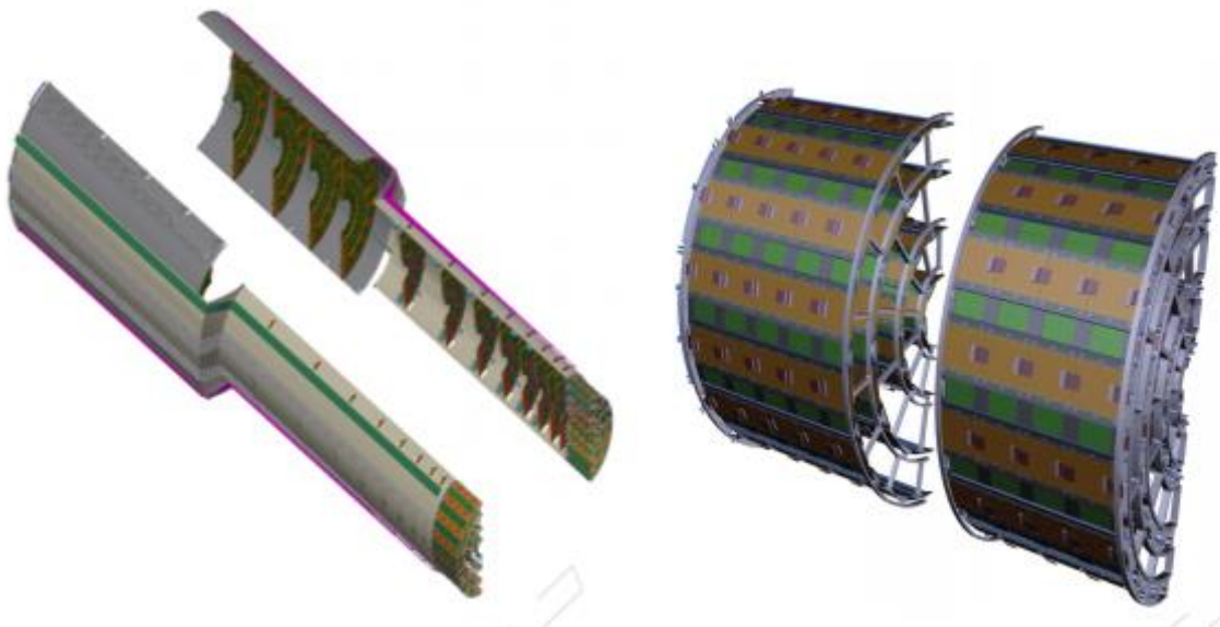
Figure 3. (Left) CAD drawings showing the split of the IT into two half cylinders per end (tdr reference fig 4.10). (Right) the two parts of the barrel split in +z (tdr reference fig 4.11)
