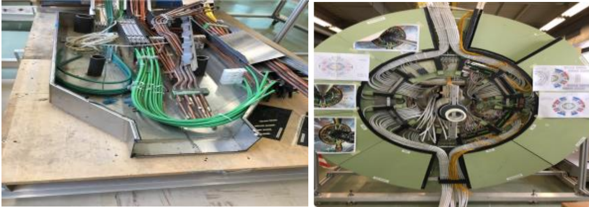
Figure 19. Pixel Phase 1 mock-up patch panels at B187. On the left, a tracker channel PP1-PP0. On the right, a picture of PP0.
