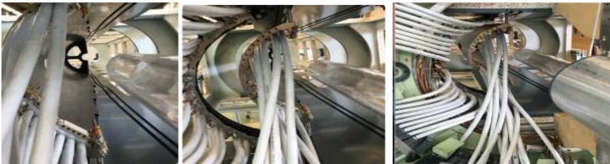
Figure 26 PP0 mock-up of Pixel Phase 1 detector services at B187.
