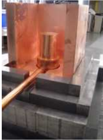
Figure 2.4: Picture of the Gator detector and its shield. The HPGe crystal is enclosed in an ultra-low background copper housing [62].
