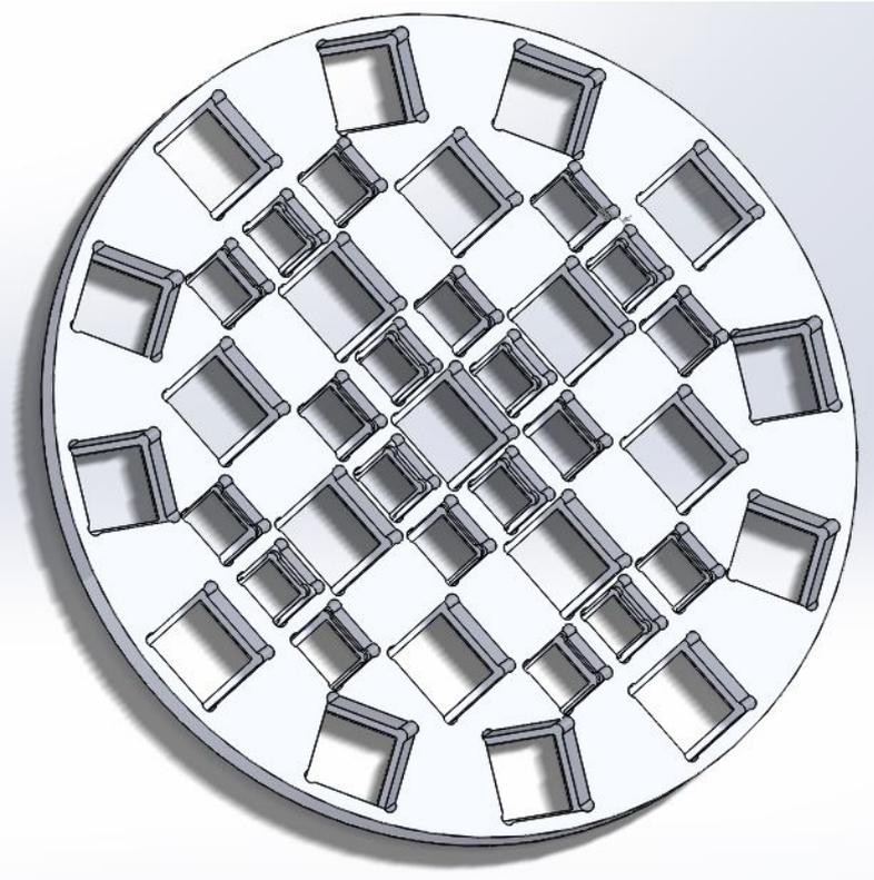
Figure 5.12: SolidWorks drawing of the top array holder for twenty-one 1-inch PMT, twelve ADP and eight  $12 \times 12 \text{ mm}^2$  MPPC.
