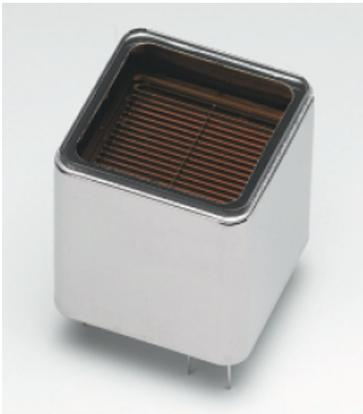
Figure 3.2: Photo of a 1-inch PMT model R8520-406. Visible are the synthetic silica window, the cobalt-free metal case and at the bottom two of the 23 pins on which the base is attached.
