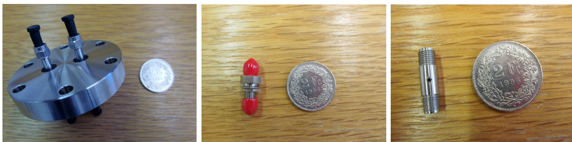
Figure 3.6: Pictures of the optical vacuum SMA feed-through (left) and SMA connectors for air (middle) and vacuum (right) that are used for the XENON1T PMT calibration setup.
