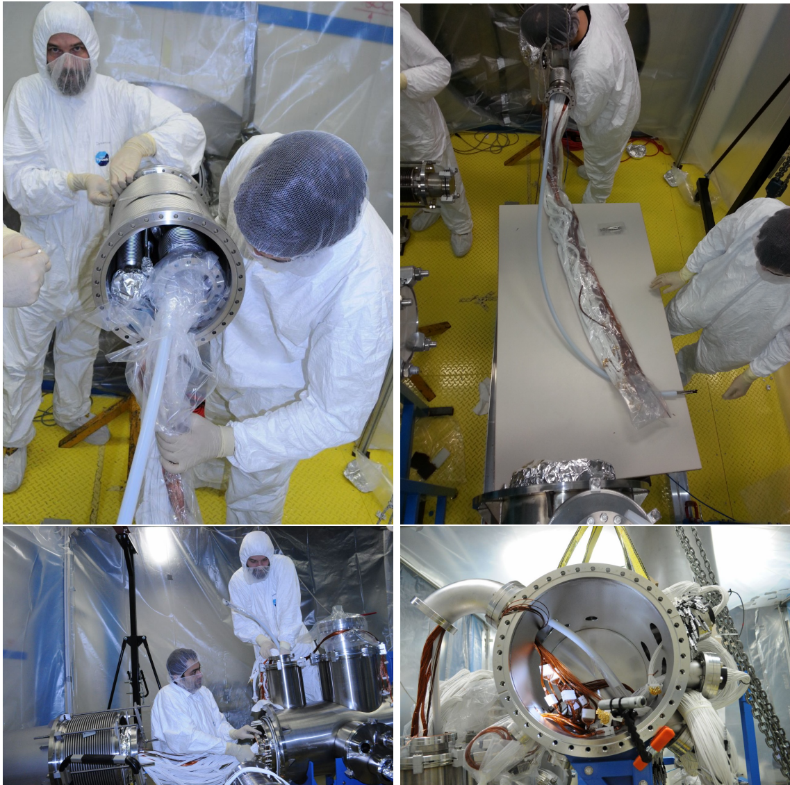
Figure 3.11: Photos from the extension of the optical fibers and cables to the vacuum feed-throughs inside the clean room built on the second floor of the XENON1T service building at LNGS.
