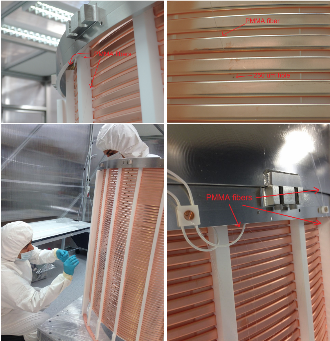
Figure 3.14: Photos from the installation of the PMMA fibers in the XENON1T TPC. The PMMA fibers used for the XENON1T PMT calibration system are 250\text{ }\mu\text{m} thick and therefore, cannot be viewed easily from the photos.
