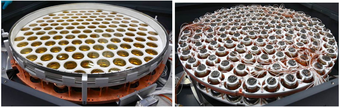
Figure 2.7: Photographs of the bottom (left) and top (right) PMT arrays after the installation of the PMTs. The PMT voltage dividing circuits and the connected signal and high-voltage cables are visible on the top array.
