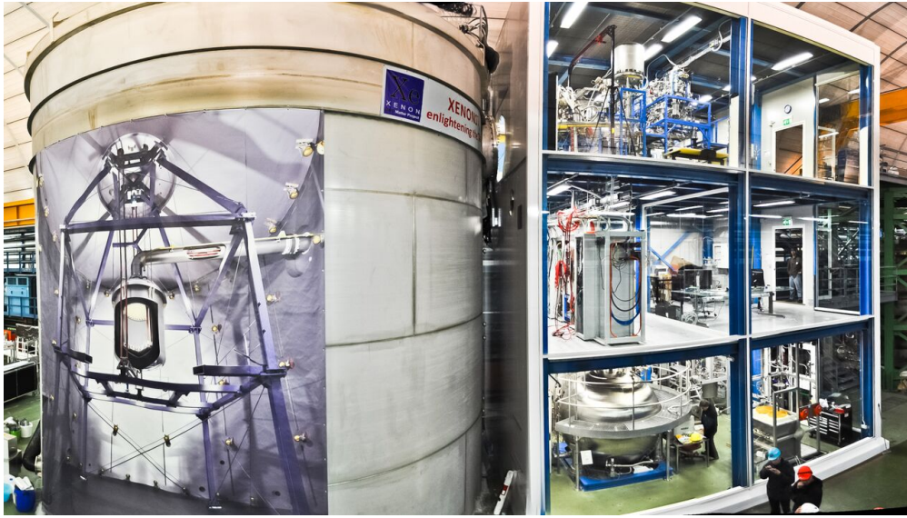
Figure 2.2: Picture of the XENON1T experiment. The water tank on the left is made of a stainless steel cylinder with 10m height and 10m diameter. An artistic drawing of the internal parts is attached to the front wall of the tank. The 3 floor service building is located on the right. The xenon storage and recovery tank is visible on the ground floor, while the DAQ system and electronics can be seen on the first floor. The cryogenic and purification systems are placed on the second floor.
