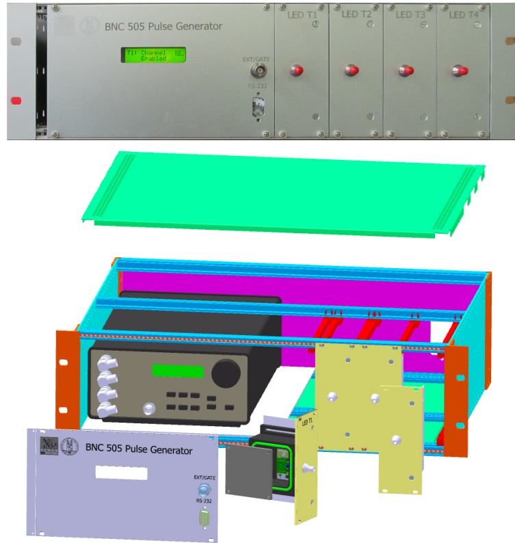
Figure 3.3: Photograph of the front side of the XENON1T LED frame with the pulse generator and the LED boxes installed (top), and a graphical model of the LED frame and its parts (bottom).
