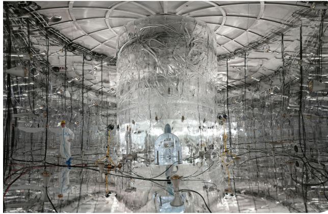
(b) After the construction of the wavelength shifting foil and the PMTs for the Cherenkov muon veto in August 2009.
