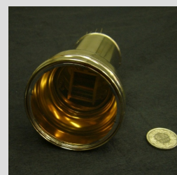
Low Radioactivity Photon Detectors (3", Total ~250)
