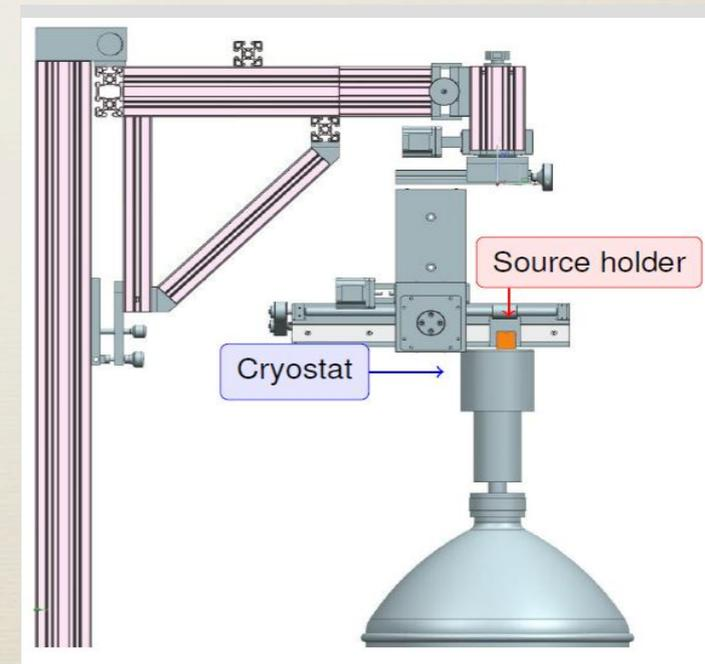
Schematic of the scanning table
