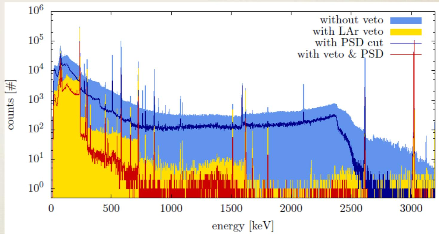
Operation of Phase II detector prototype in LArGe:
