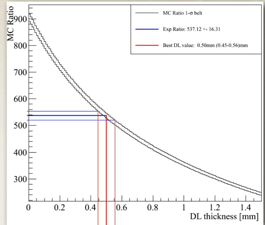
Active volume determination using  $^{60}\text{Co}$ : count rate under the peaks @ 1173.2 keV and 1332.5 keV is compared to the simulated one.
