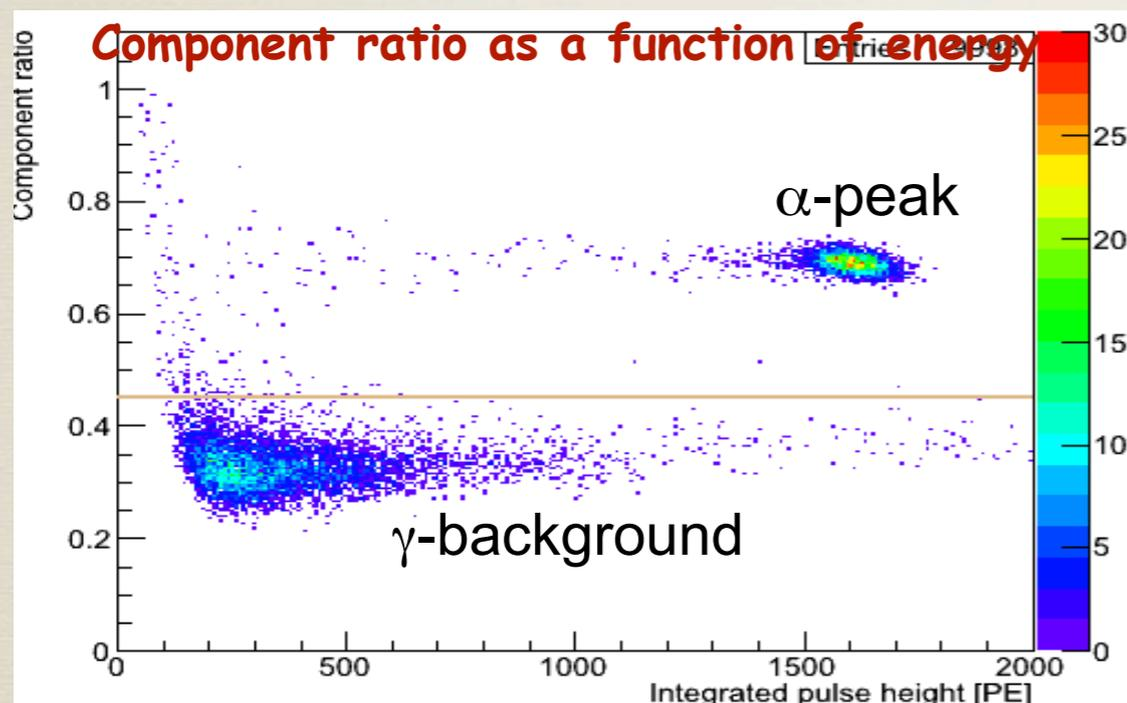
**Component ratio:** Is the integral in the fast component over the integral of whole trace.
