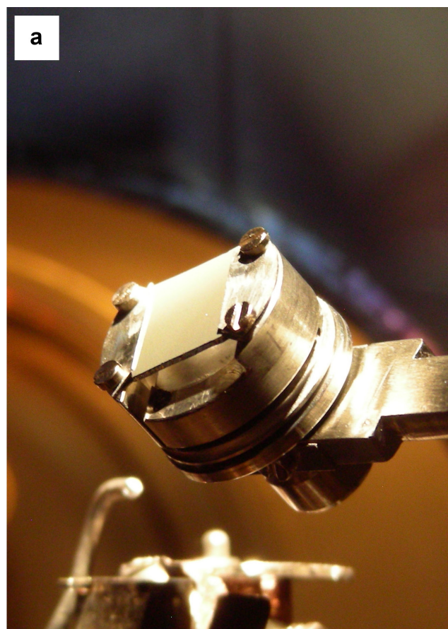
Extended Data Figure 1 | Thermal desorption spectroscopy. a , h-BN/Rh(111) thin-film sample and sample holder ready for the desorption experiment in the ultrahigh-vacuum chamber. b , Thermal desorption experiment with temperature and power data shown in the top panel and pressure data in the bottom panel. The purple data are pyrometer readings,
