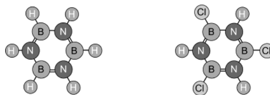
Figure 1. Sketches of the two molecules borazine (HBNH) 3 and B-trichloroborazine (CIBNH) 3 that are used for the synthesis of h -BN/Ni(111).
