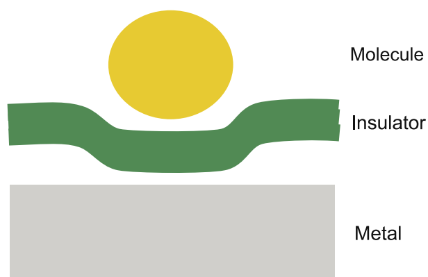
Fig. 1. Schematic side view of a single layer dielectric (insulator) on top of a metal. The dielectric strongly changes the properties of adsorbed molecules as compared to the case without dielectric. If the dielectric corrugates, the structures may be used as templates on which single molecules may be laterally ordered.
