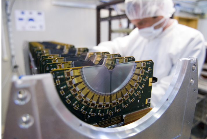
Figure 4.50: Photograph of one half of the VELO detector during its assembly in the clean room [187].
