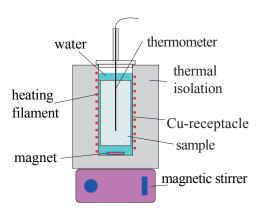
In a vessel, which is thermally isolated and which possesses a small heat capacity W, the metallic sample is heated in a water bath. Electric energy is provided by an external power supply . . .
